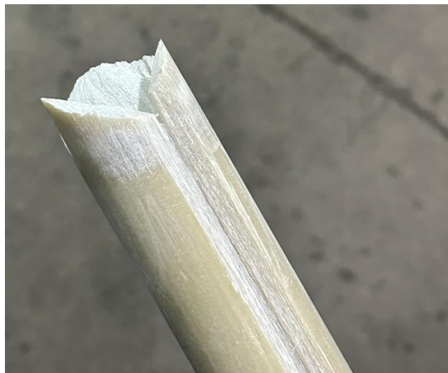
Figure 3: Example of Radial Crack from Compression
