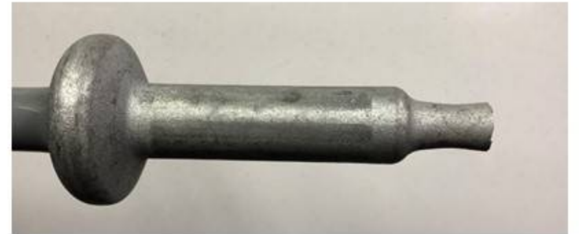
End Fitting Break
