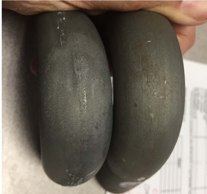
Figure 2.3 MacLean TDG bolts after bend
