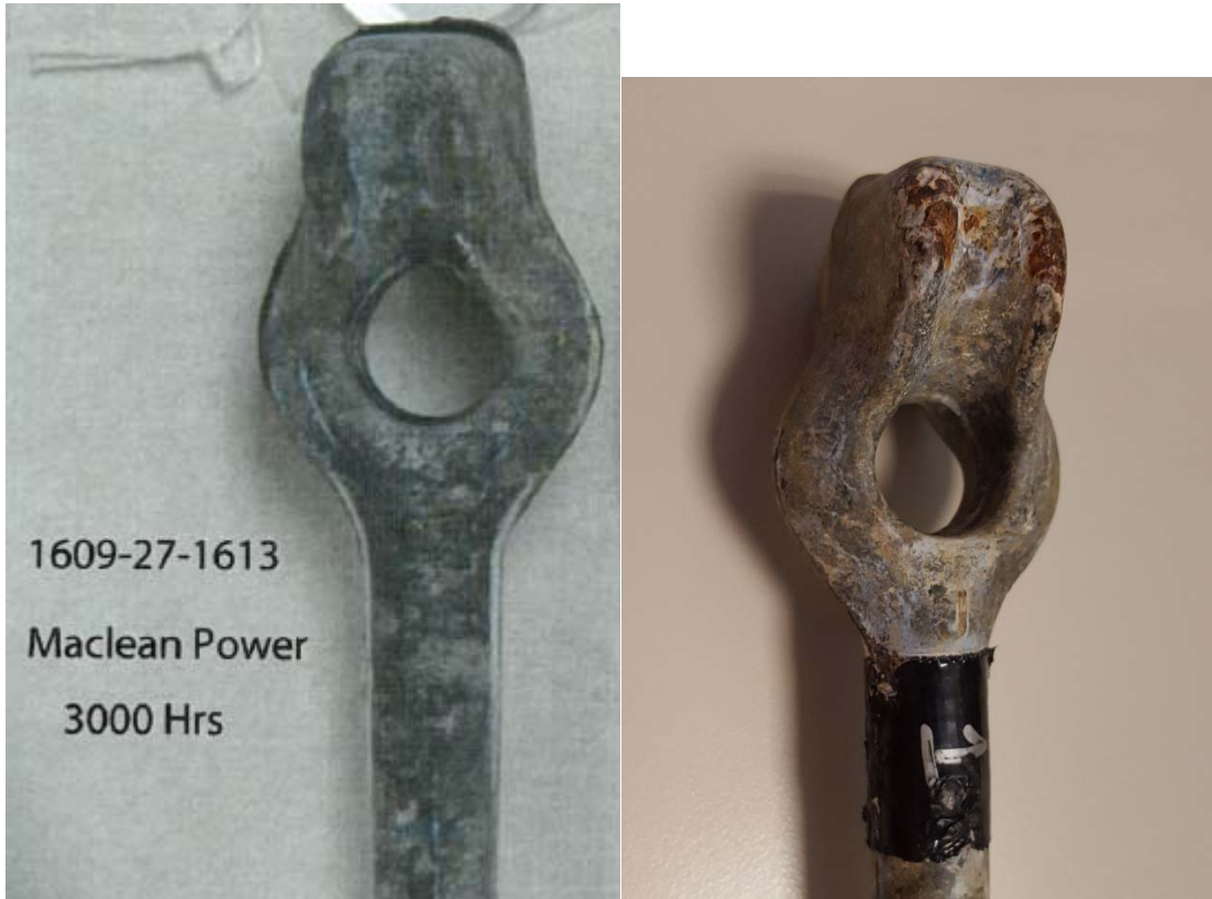
Figure 1.1: J8052-T after 3000 Hours Salt Spray and 4000 Hours Salt Spray (right)
