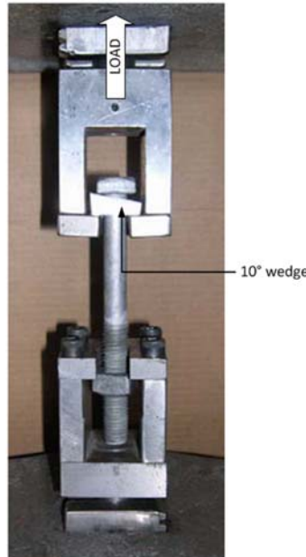
Figure 2.1: Tensile test set up (apparatus used: Instron #300DX-C3A).
