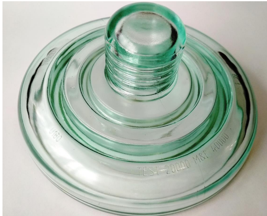
Fig. 10 – Completed Insulator Shell
