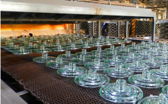
Fig. 8 – Thermal Cycle – heated up to 300 C
