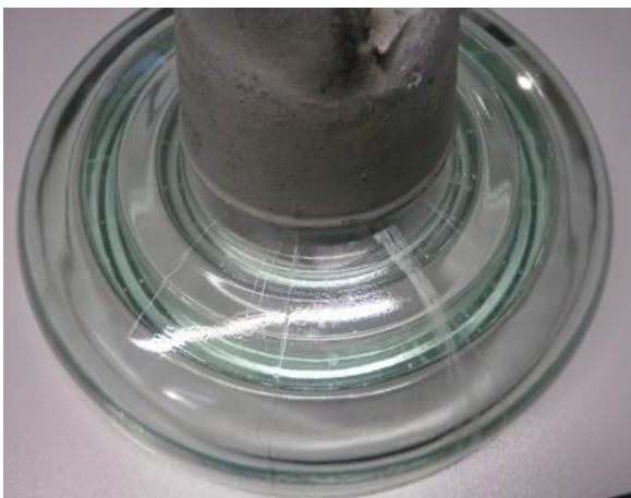
Fig. 13 – Electrical Flash-over Test
