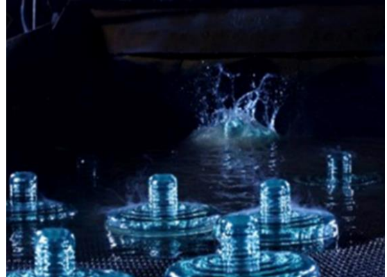
Fig. 9 – Thermal Shock – water cooled -120 C
