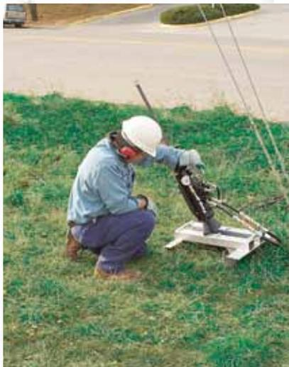
③ Use the Load Locker to pull test the anchor.
